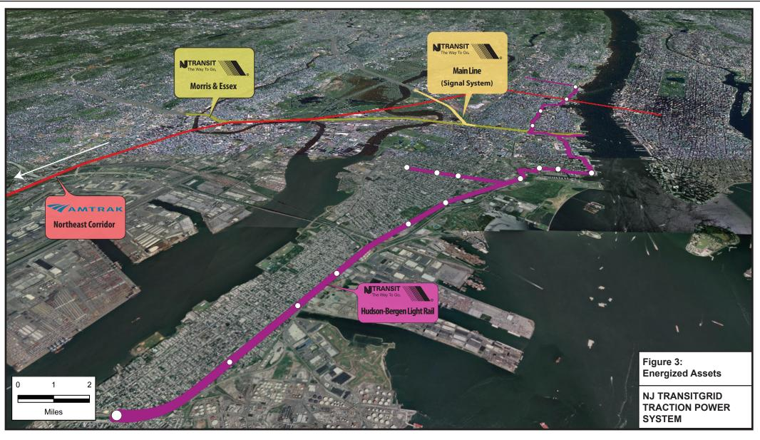
Note: Energized assets will also include some non-traction loads including: Hudson Bergen Light Rail stations, Hoboken Terminal, and other signal power, tunnel ventilation, pumping, and lighting loads.
